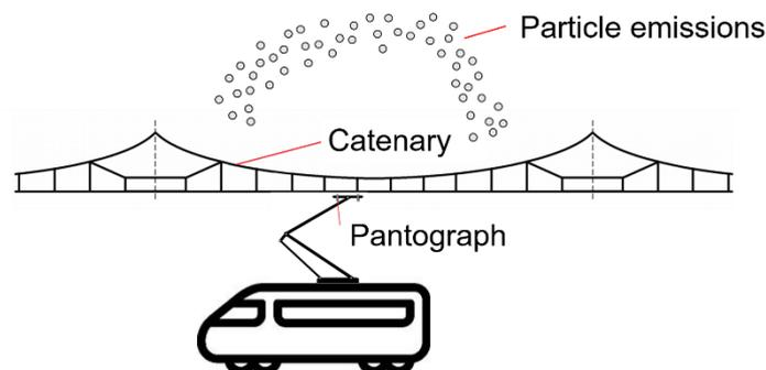
Figure 1. Sketch of the railway catenary–pantograph system including illustration of wear particle emissions
